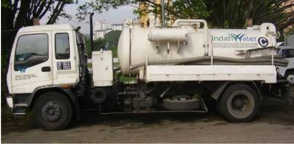
Figure 34: Vacuum truck in Malaysia
